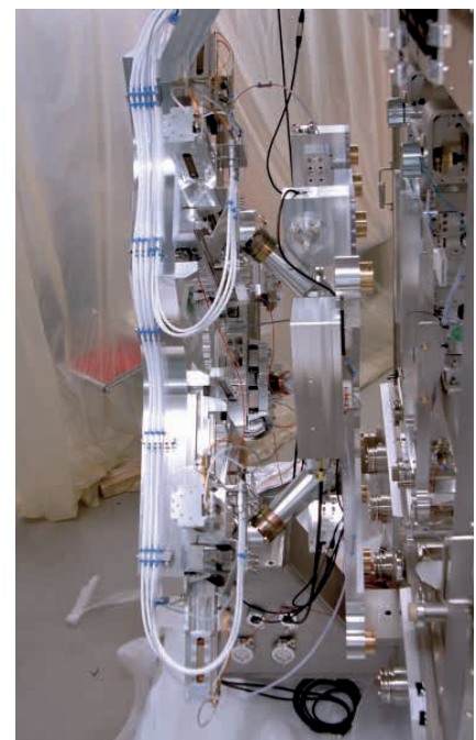
Automated sandwich pick-and-place machine for large area films in HV to 10^{-6} hPa. The parallel-kinematic SpaceFAB positions on 6 axes and is distinguished by its low profile
