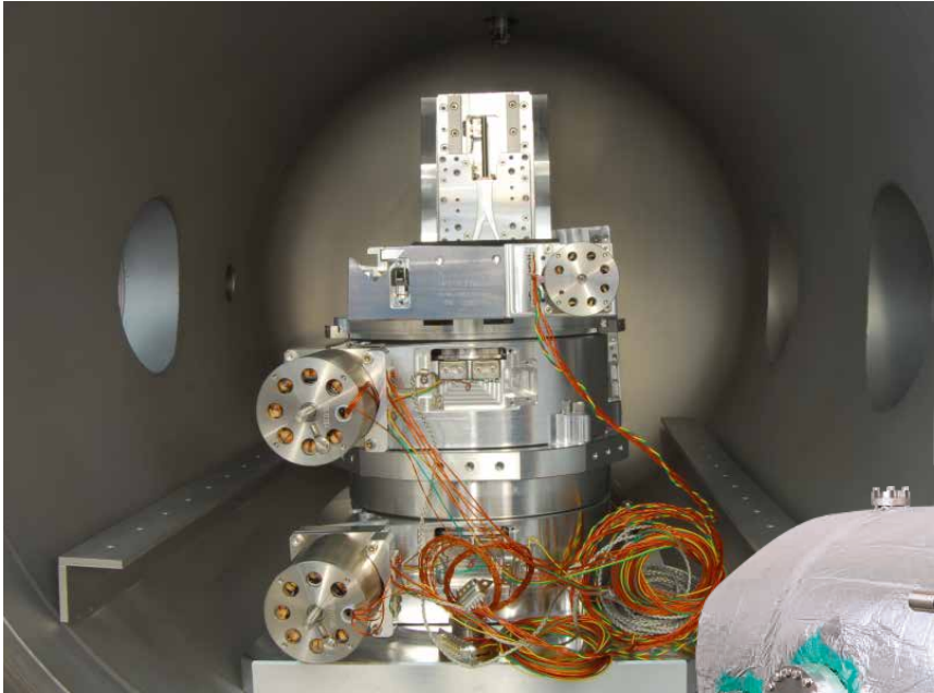
View in the vacuum chamber. Here, a multi-axis design awaits start-up and outgassing measurement
