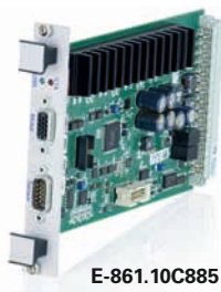
E-861.10C885 Motion controller module for NEXACT® piezomotor systems
