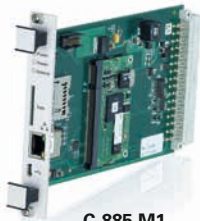
C-885.M1 Digital processor and interface module
