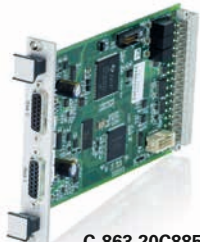
C-863.20C885 Motion controller module for DC motors
