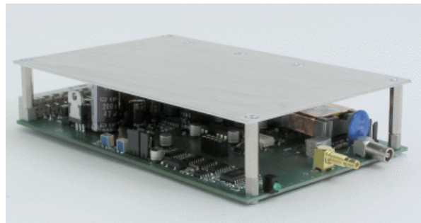
Fig. 2: E-617.00F high-power piezo amplifier OEM module
