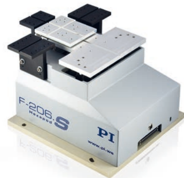
Constant strut-length Hexapod design. The drive units move the joint position up and down affecting the linear and rotary position of the platform
