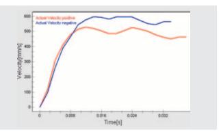
PlLine<sup>®</sup> ultrasonic linear motors provide excellent dynamic properties. They provide acceleration to several g and can achieve step-and-settle of a few 10 microseconds for small distances
