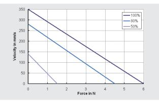
Force / velocity motor characteristic of a PILine® motor 6 N holding force. The percentages refer to the control signal level, which denotes the coupling of the electric power of the actuator
