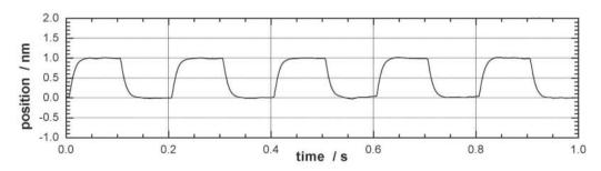
Sequence of open-loop 1 nm motions of a NEXLINE® drive
