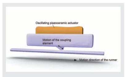
The piezoceramic actuator is excited to ultrasonic vibrations with a high-frequency AC voltage between 100 and 200 kHz. The deformation of the actuator leads to a periodic diagonal motion of the coupling element to the runner. The created feed is roughly 10 nm per cycle; the high frequencies lead to the high velocities
