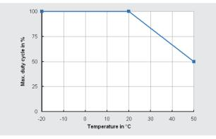
Maximum duty cycle depending on the ambient temperature with a control signal level of 100\%  $\,$
