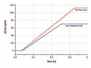
Constant velocity and smooth driving of a NEXLINE® drive are best achieved in nanostepping mode, but the maximum attainable velocity is higher in full-step mode
