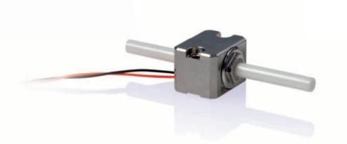
PIShift drives are space-saving and cost-efficient piezo-based drives with relatively high holding forces of up to 10 N and a basically unlimited travel range. They make use of the stick-slip effect (inertia effect) – a cyclical alternation of static and sliding friction between a moving runner and the drive element generated by the piezo element – for a continuous feed of the runner. With an operating frequency above 20 kHz, PIShift drives reach velocities of more than 5 mm/s.
