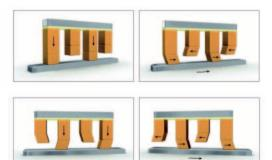
Motion sequence of a NEXLINE® actuator
