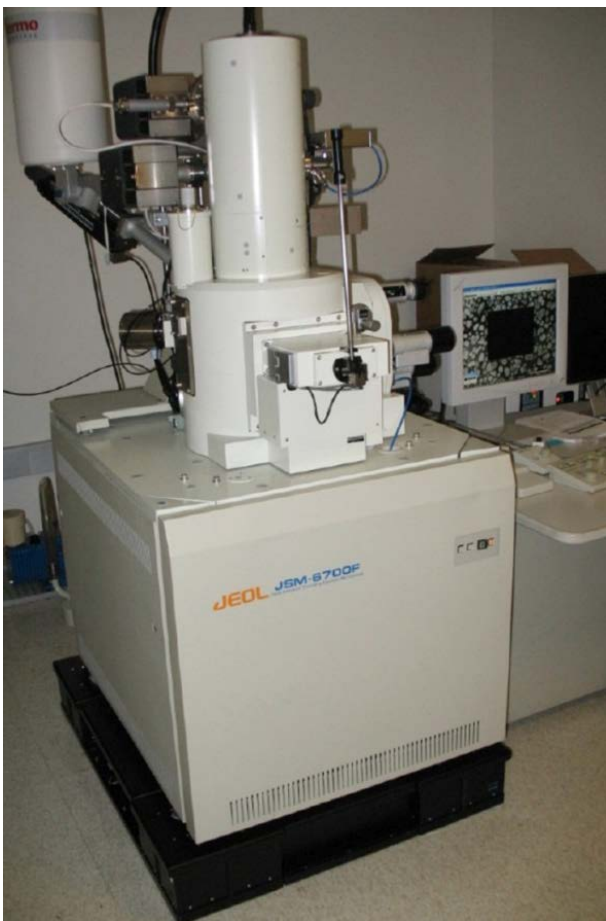
Fig. 4 STACIS isolation is also possible for smaller equipment, e.g. for scanning electron microscopes (image: TMC)
