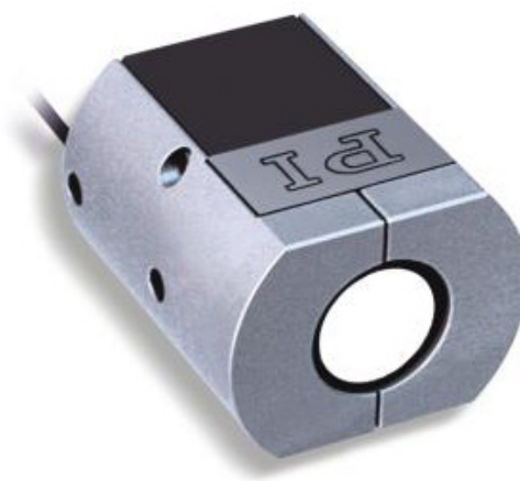
Fig. 3 Compact piezo tip/tilt mirror with two orthogonal axes and 100 mrad optical deflection angle with 0.0005 mrad resolution; length 38 mm
