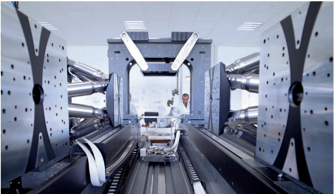
This 20-ton, 56-axis motion system is used for x-ray microscopy and quality assurance of x-ray optics. It is equipped with 56 motors, 16 controllers, 7 air bearing granite sliders and has an overall mass of more than 20,000 kilograms. An extraordinary precision of some hundreds of nanometers over the full range could be achieved.
