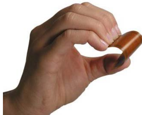
Fig. 6 Bending radii of up to 20 mm can be easily realized with DuraAct patch transducers
